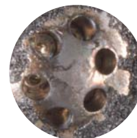
Injector after one P.i. treatment.
